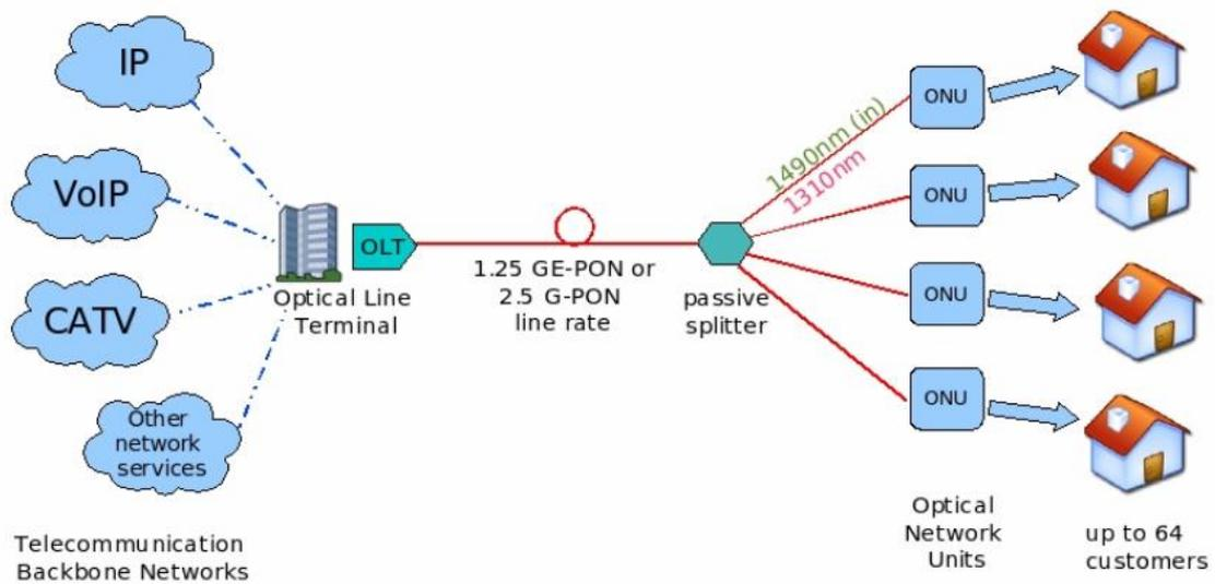
Fig. 2 GPON Ethernet Passive Optical Network
