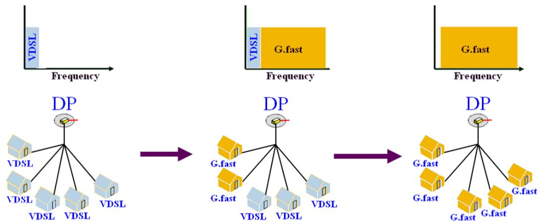
Fig. 3xDSL and G.Fast coexistence
