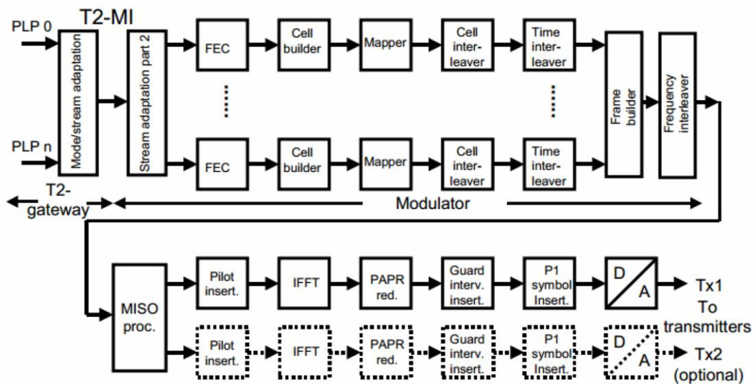
Figure 2 DVB-T2 System Architecture
