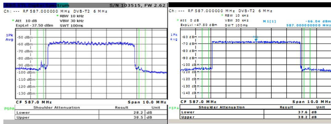
Figure 8 DVB-T uses different subcarriers 8k (left), 32k (right) mode
