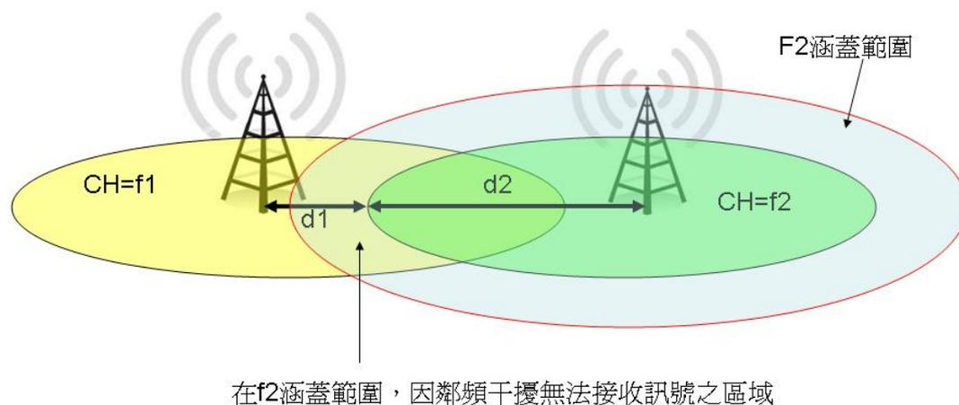
Figure 10 Adjacent channel interference schematic diagram
