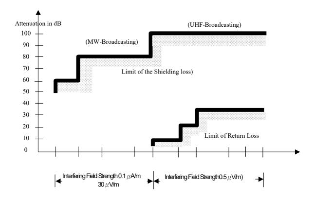
Figure 2 Shield room with absorbers for shielding loss and wall return loss requirements
