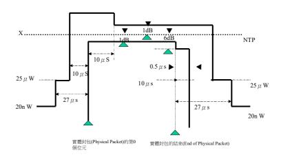
This requirement shall apply except when p0 of the next transmitted packet occurs less than  $54\mu s$  after the end of the transmitted physical packet. The power level of X shall be less than 315mW, and also shall be less than dB(NTPm)+4dB.
