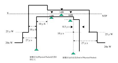
The power level of X shall be less than 315mW, and also shall be less than NTP+4dB.
