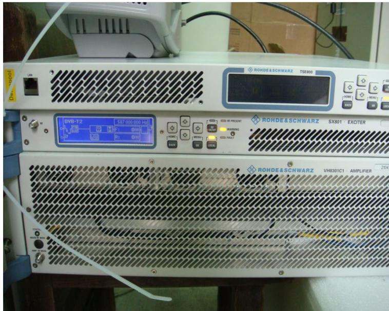
Figure 5 DVB-T2 transmitter encoder, actuators and power amplifier
