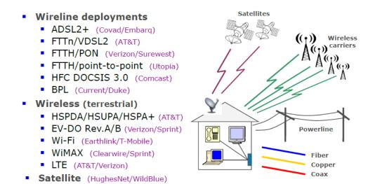
Fig. 1 Broadband access techniques and service providers in USA
