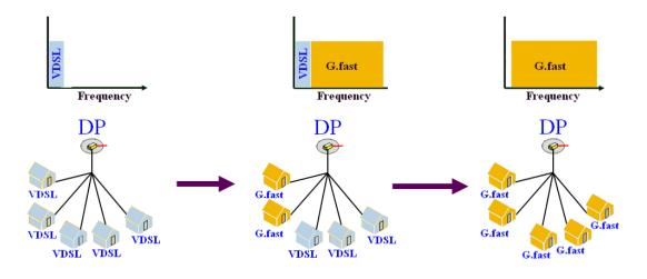
Fig. 3xDSL and G.Fast coexistence
