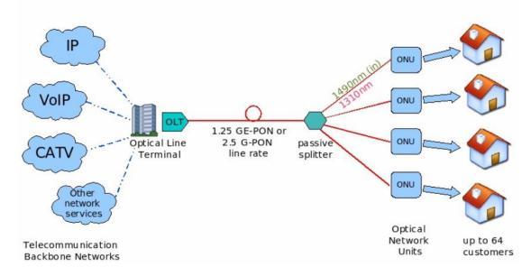
Fig. 2 GPON Ethernet Passive Optical Network
