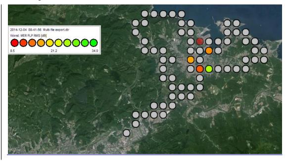
Figure 9 PLP1 modulation error rate of DVB-T2 mobile receive
