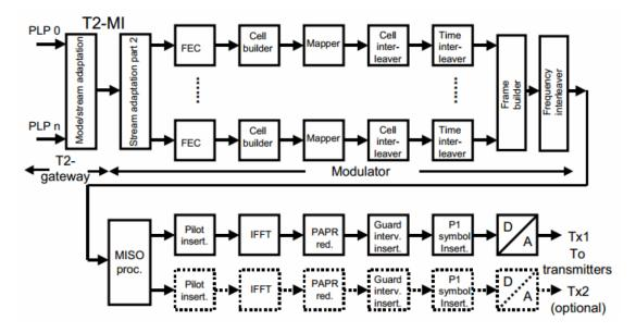
Figure 2 DVB-T2 System Architecture
