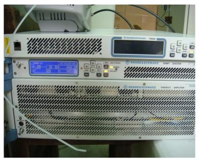
Figure 5 DVB-T2 transmitter encoder, actuators and power amplifier
