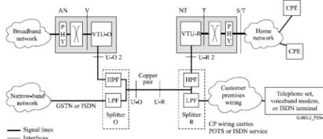
Figure 5-4 G.993.2 - Generic application reference model for remote deployment with splitter
